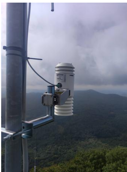
Fig. 2: Instrument AQT530 from Vaisala on the tower top of Milešovka observatory.
