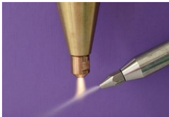
Fig. 1: Mixing of the plasma stream and the CO 2 snow spray
