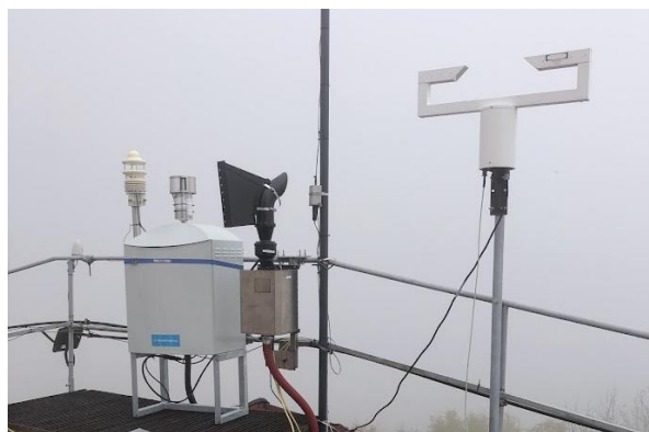
Figure 1. Measurement set-up at the Milešovka station: CDA, FM-120, and PVM.
