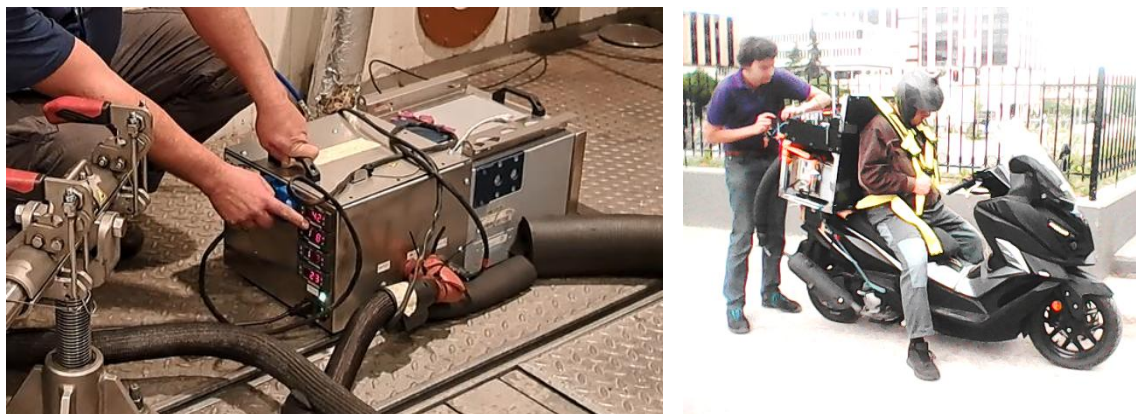
Fig. 1: Mobile FTIR analyzer in the test cell (left) and mounted on a motorcycle (right).
