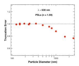
Fig. 1 Truncation error of CAPS  $PM_{SSA}$  at 630 nm measured using non-absorbing PSLs.
