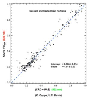
Figure 2. Comparison of measured SSA using CAPS  $PM_{SSA}$  (630 nm) and CRD Extinction+Photoacoustic Absorption Spectrometer (courtesy of C. Cappa, U.C. Davis) operating at 532 nm.
