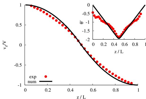
Figure 1: Nondimensional axial velocity and gradient (inset) along the centerline.
