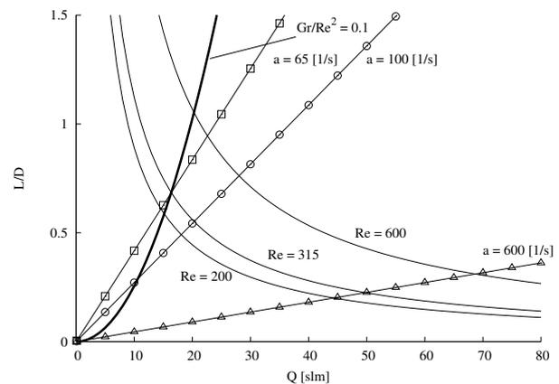
Figure 2: Operation map for the counterflow with nozzle diameter 25 mm. The Reynolds number is defined using half of the separation, the exit velocity, and the nitrogen kinematic viscosity:  $Re = V(L/2)/\mu$ .
