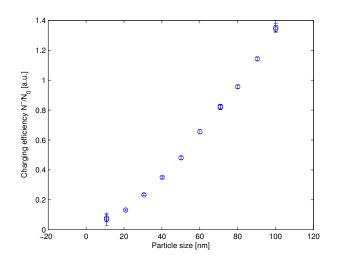
Figure 1: The size dependency of the charging efficiency of the indirect photoelectric diffusion charger for a spark discharge aerosol (GFG 1000, Palas, Germany).
