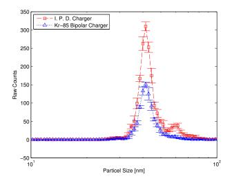
Figure 2: A comparison between the indirect photoelectric diffusion charger and a new Kr-85 bipolar charger (350 MBq) for a 41 nm spark discharge aerosol measured by a SMPS.
