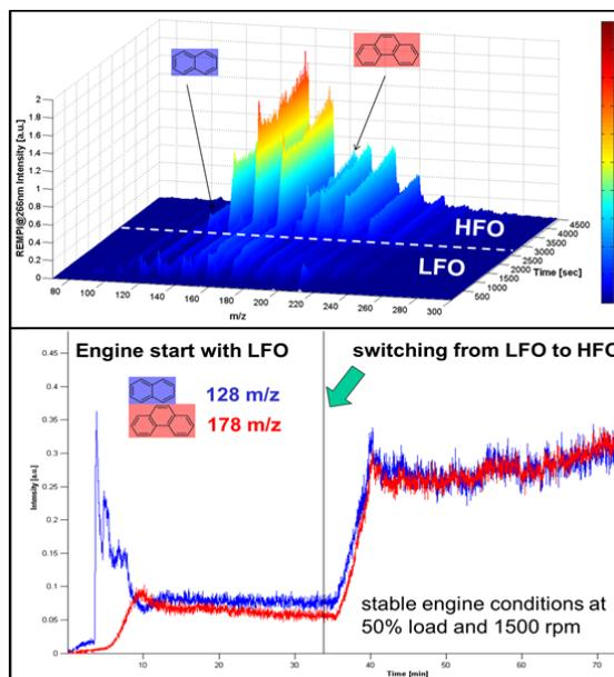
Figure 2 On-line measurement of the gas-phase aromatics (PAH and alkylated-PAH) in combustion aerosol from a **ship diesel engine** operated with distillate fuel (light fuel oil, LFO) and residual fuel (heavy fuel oil, HFO) top) 3D-representation of the changes in aromatic REMPI mass spectral signature over time during a switch from “clean” LFO -fuel to “dirty” HFO-fuel. The lower part of the figure depicts the time-intensity curves for 2 selected PAH, naphthalene and phenanthrene.,
