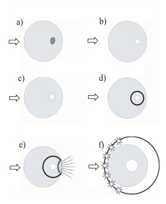
Figure 1. Optical breakdown on liquid droplet.
