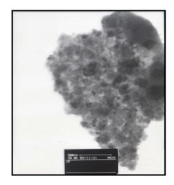
Figure 1. TEM photograph of the fresh nanosized  $\mbox{Cu}/\gamma\mbox{-}\mbox{Al}_2\mbox{O}_3$  catalyst.
