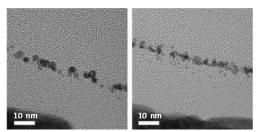
Figure 1. Cross-sectional TEM images of the OLEDs incorporating the Au NPs fabricated using the SDG-ESP (left) and VTE (right).
