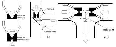
Fig. 1 Schematic diagram of the collision systems
