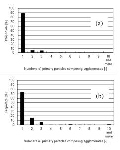
Fig. 2 Distributions of the number of primary silica particles composing the respective agglomerates after the collisions
