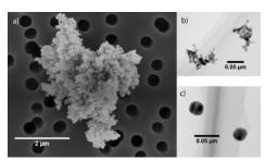
Figure 1. a) Typical emitted agglomerate with nanostructures related to sintered particles. b) Aggregates formed by the SDG. c) Sintered particles
