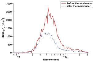
Figure 1- Size distribution measured before and after the thermodenuder at 200 °C
