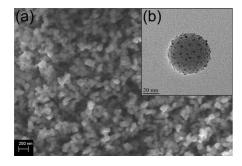
Figure 1: (a) An SEM image of the decorated particles on a glass substrate after a collection time of 30 min and (b) a TEM image of a single particle.
