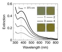
Figure 2: Extinction spectra of the multilayered nanoparticle structures with 1–4 layers. The inserts show photographs of the samples.
