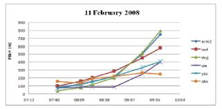
Figure 1. Hourly trend of PBL height in Milan for February 11<sup>th</sup>, 2008. The figure shows the five parameterizations as well as the observed data by balloon sounding.
